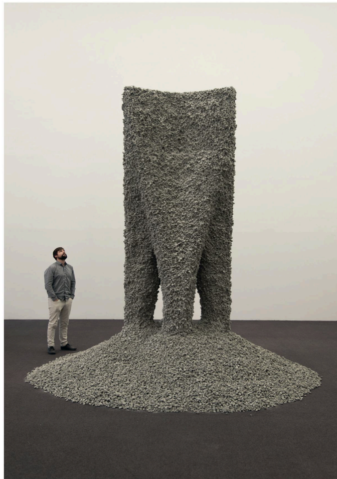
A four-metre tall, load bearing column out of a pile of rocks and a string [12]
